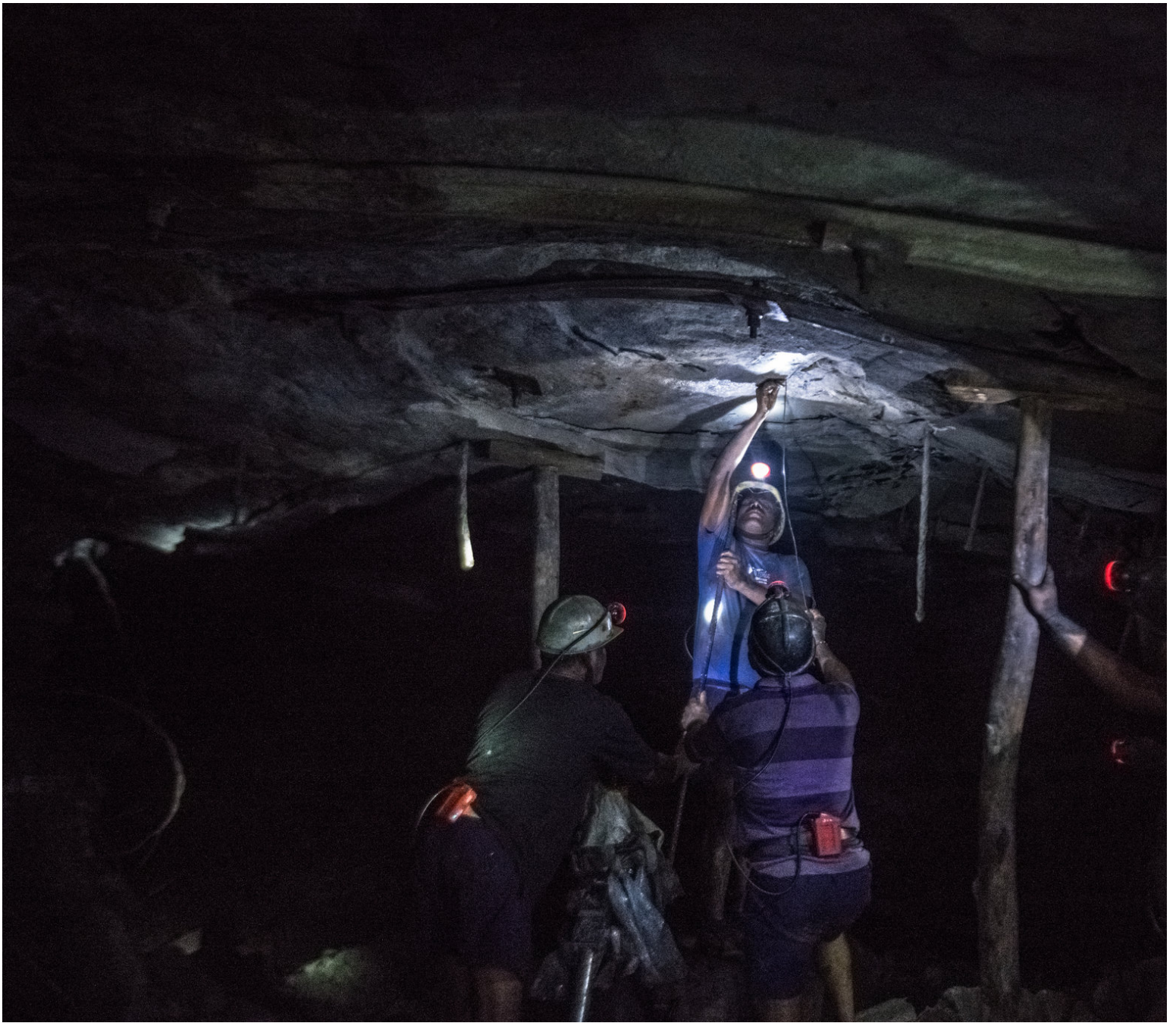
Miners reinforced the roof of a coal pit in Telangana. Rebecca Conway for The New York Times
